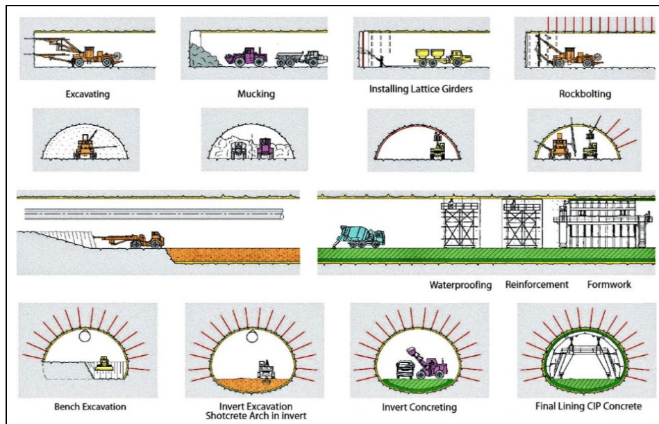
159 Fig. 10. NATM tunnel excavation stages from [8] ASG, 2010.
