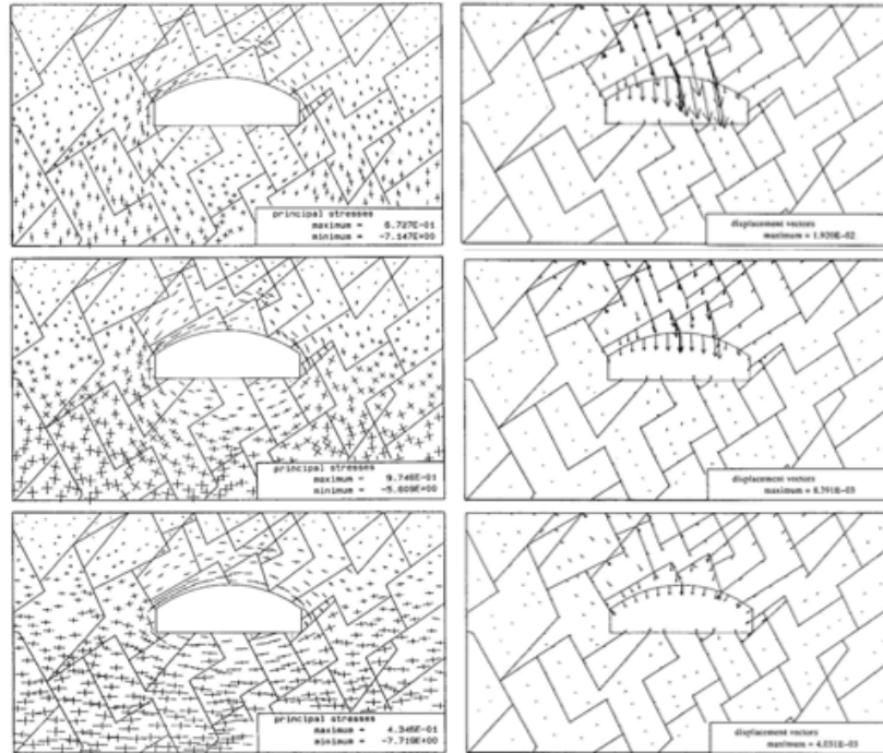
Fig. 31. Scoping studies with UDEC-BB show the positive effect of higher horizontal stress. With continuum modelling such improvement is in doubt.
