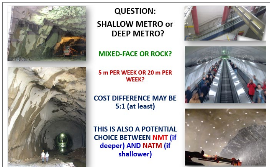
210 Fig. 16. Shallow metro consequences: mixed-face, overbreak, collapse? 211
